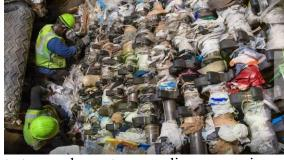
(Caption: This photo illustrates workers at a recycling processing plant climbing up onto the equipment to cut away and remove plastic bags, cords, hoses and other items since they get tangled and stop the machinery from functioning. This slows down the manufacturing process and places a burden on both the recycling facility and the workers.) Please DO NOT put the following materials into the recycling cart: liquids, food, waste, fabric, wood, hoses or cords, styrofoam or plastic bags.
