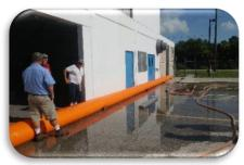
flood barrier (orange tube) being tested at the Water Treatment Plant. The barrier test was successful and should help protect the building from flooding.
