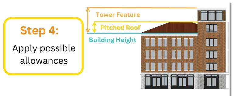
Architectural features constitute height allowances, which are parapet walls (10 feet additional allowance), pitched roof forms (12 feet additional allowance), rooftop amenities (10 feet additional allowance with conditions), and a tower feature (20 feet additional allowance with conditions). The maximum allowance to overall building height cannot exceed 20 feet.
