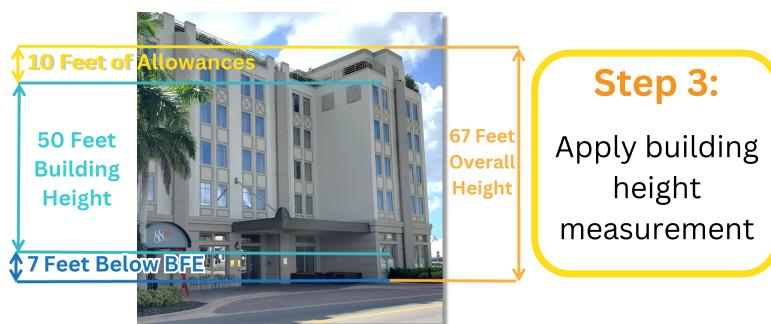
The zero-foot height measurement is taken from Design Flood Elevation (Base Flood Elevation [BFE] plus required freeboard) in accordance with the Florida Building Code. Areas below BFE are limited to storage, parking, and access.
