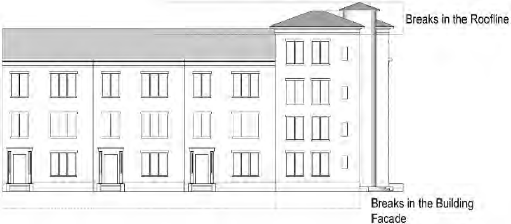
Figure 5: Breaks in the Building Façade
