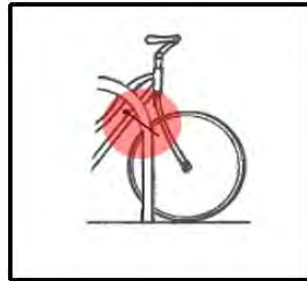
Figure 10.13(b)(1): U-lock secures the bicycle frame and one wheel to the rack
