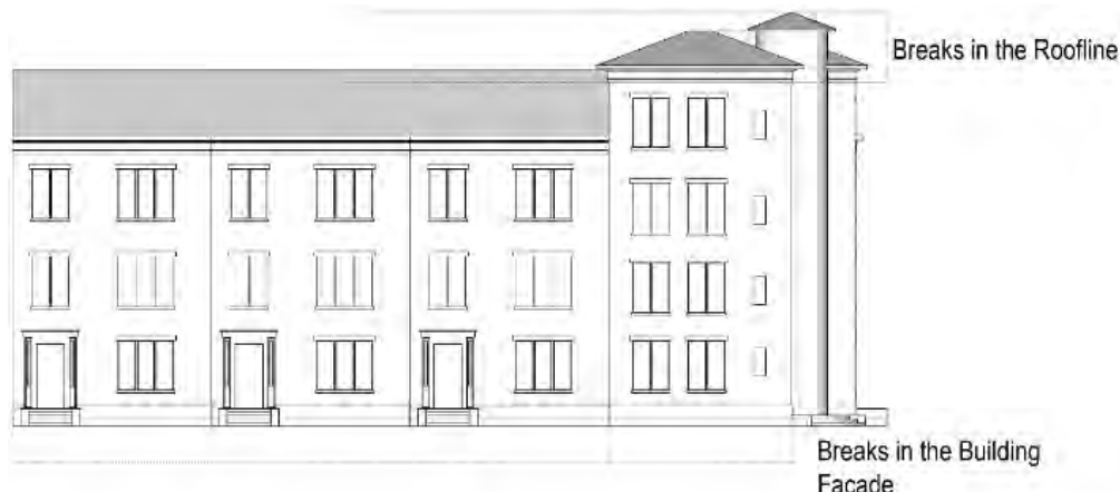
Figure 5: Breaks in the Building Façade
