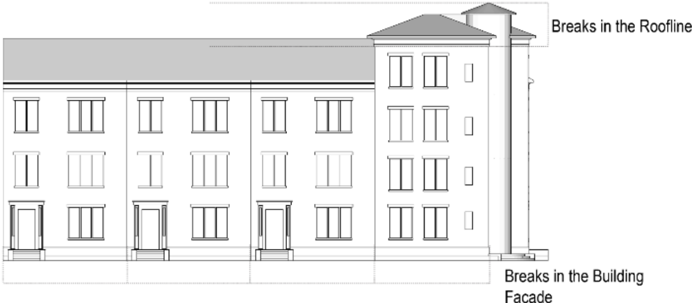
Figure 5: Breaks in the Building Façade
