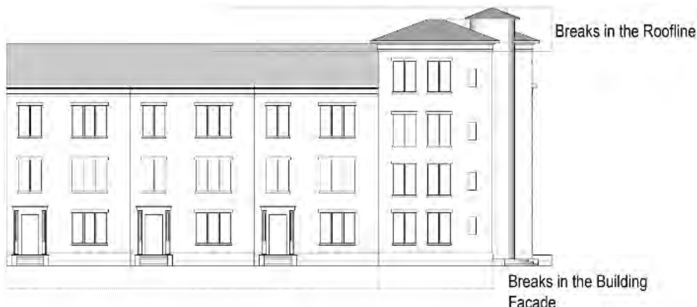
Figure 5: Breaks in the Building Façade
