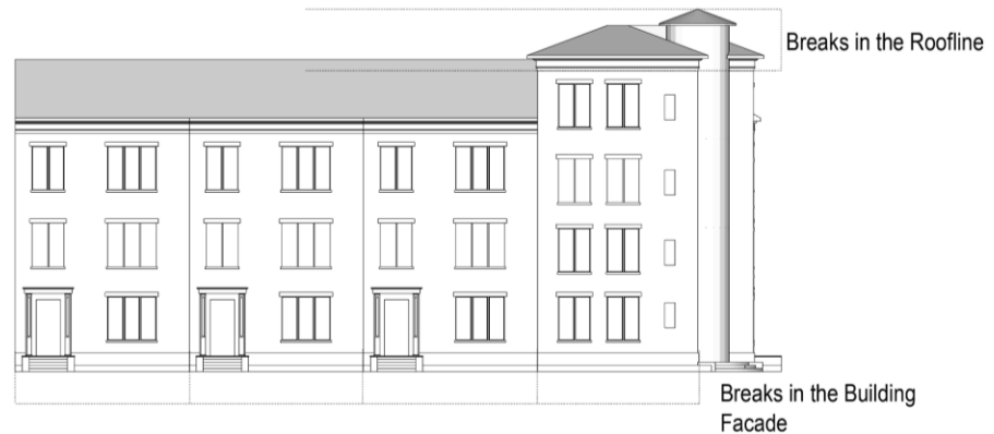
Figure 5: Breaks in the Building Facade
