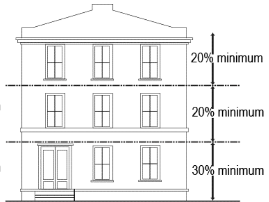
Figure 17: Façade transparency requirement for buildings without shopfront
