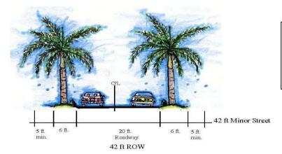
Design speed: 15 mph Right-of-way width: 42 feet Curb radius: 15 ft
