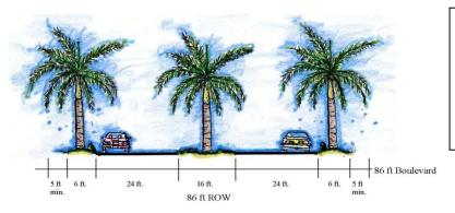
Design speed: 30-35 mph Pavement width: 24-16-24 feet
