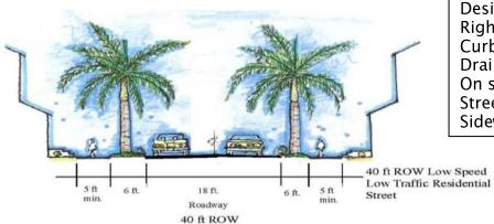
Design speed: 10-15 mph Right-of-way width: 40 feet Curb radius: 10 ft
