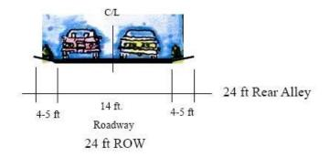
Design speed: 10 mph Right-of-way width: 24 feet Curb radius: 5 ft
