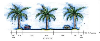
Design speed: 20–30 mph Pavement width: 20–14–20 feet
