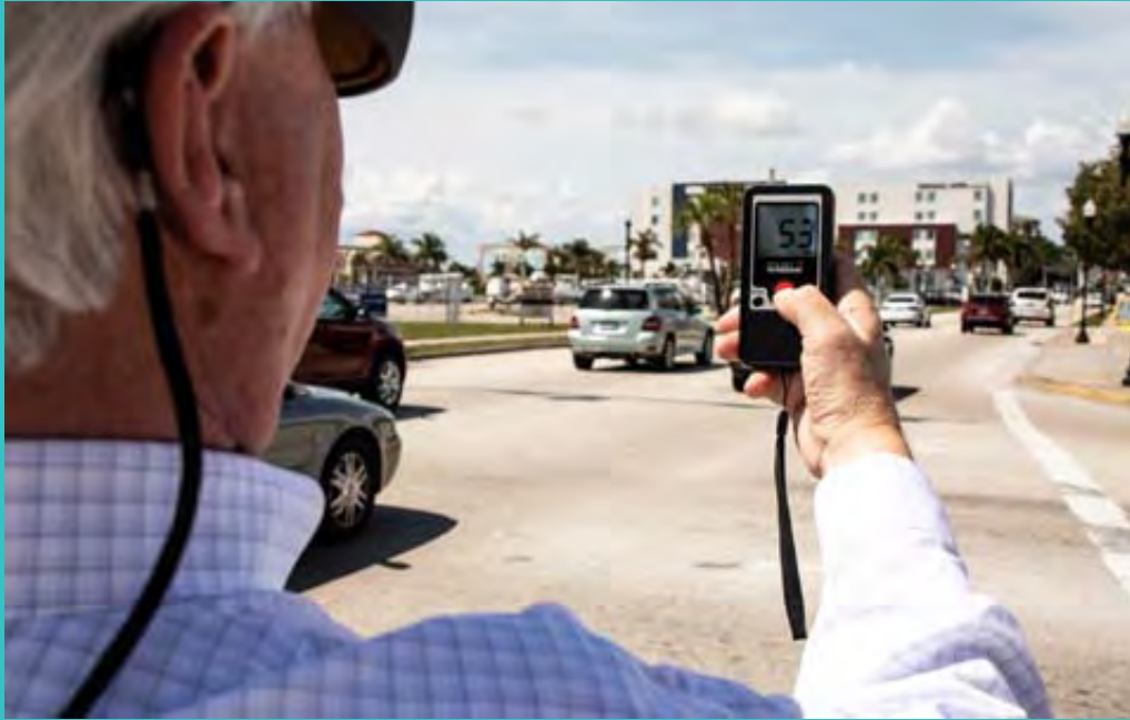
Transportation Planner Rick Hall Measuring Vehicle Speeds of 53 mph on US 41 in Downtown
