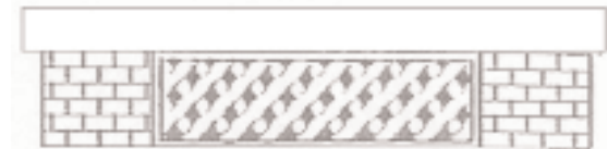
Appropriate: wood lattice infill between brick piers
