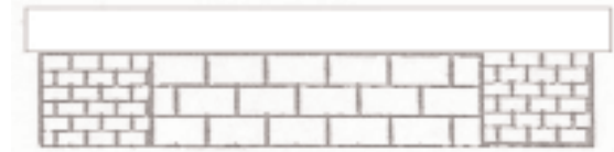
Inappropriate: continuous concrete block infill
