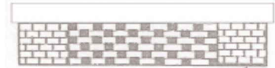
Appropriate: pierced continuous brick infill
